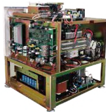
32kW / 40kW Super Capacitor Bank (PSU Generator)
