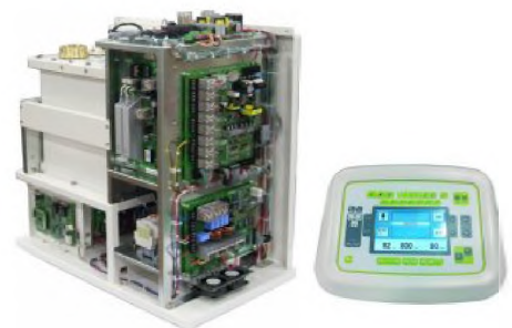
50KW generator and LCD OP console
